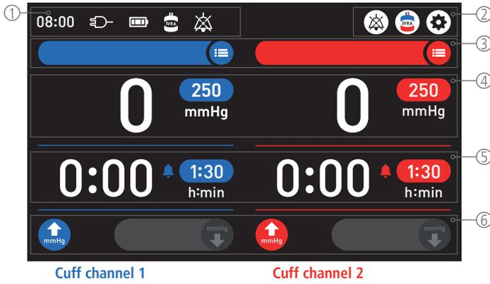
The main screen is divided up into ① status bar, ② control bar, ③ channel bar, ④ pressure display, ⑤ time display and ⑥ inflation / deflation area.
