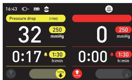
An error is displayed in the channel bar. The cuff channel to be tested alternates between yellow and the channel colour.
