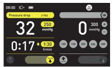
An error is displayed in the channel bar. The cuff channel alternates between yellow and the channel colour
